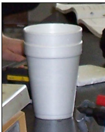
The Simple 2-Cup Calorimeter
